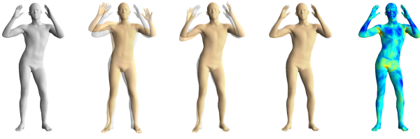
Figure 8: Qualitative visualisation of input shape (gray) projected onto model in Fig. 1 with (cols 2-4) J = 5, 11, 17 dimensions. Col 5 shows residual energy of projection with J = 17 .
