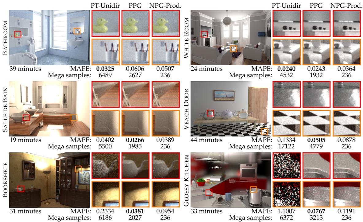
**Figure 8.16:** Equal-time comparison of unidirectional path tracing (PT-Unidir), practical path guiding (PPG), and our product-driven neural path guiding (NPG-Product). Despite the large computation cost of NPG, it performs competitively with PPG and unidirectional path tracing in scenes with difficult light transport (bottom two rows, sorted by difficulty in ascending order).
