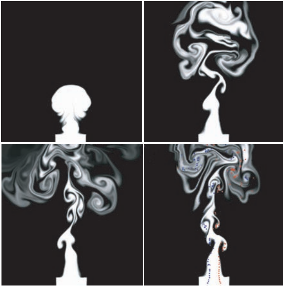
Figure 5: Rising Smoke in 2D generated by our method. Even with the small number of computational elements (200 vortex particles in this case), it can express a complex, swirling movement of the gaseous phenomena.
