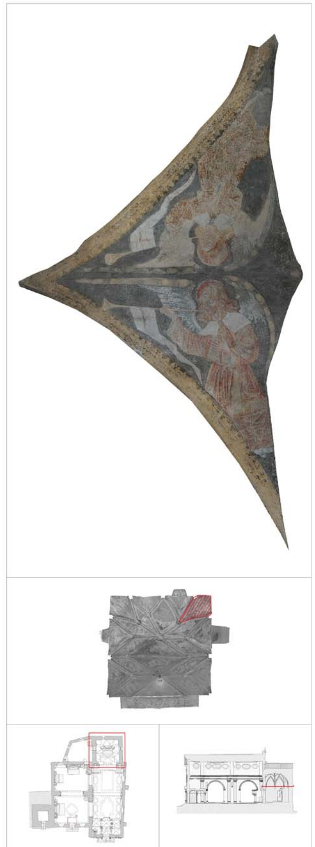
Fig. 7. Unrolled 2D measurable orthophoto of the wall painting with marked position in the architecture plan
