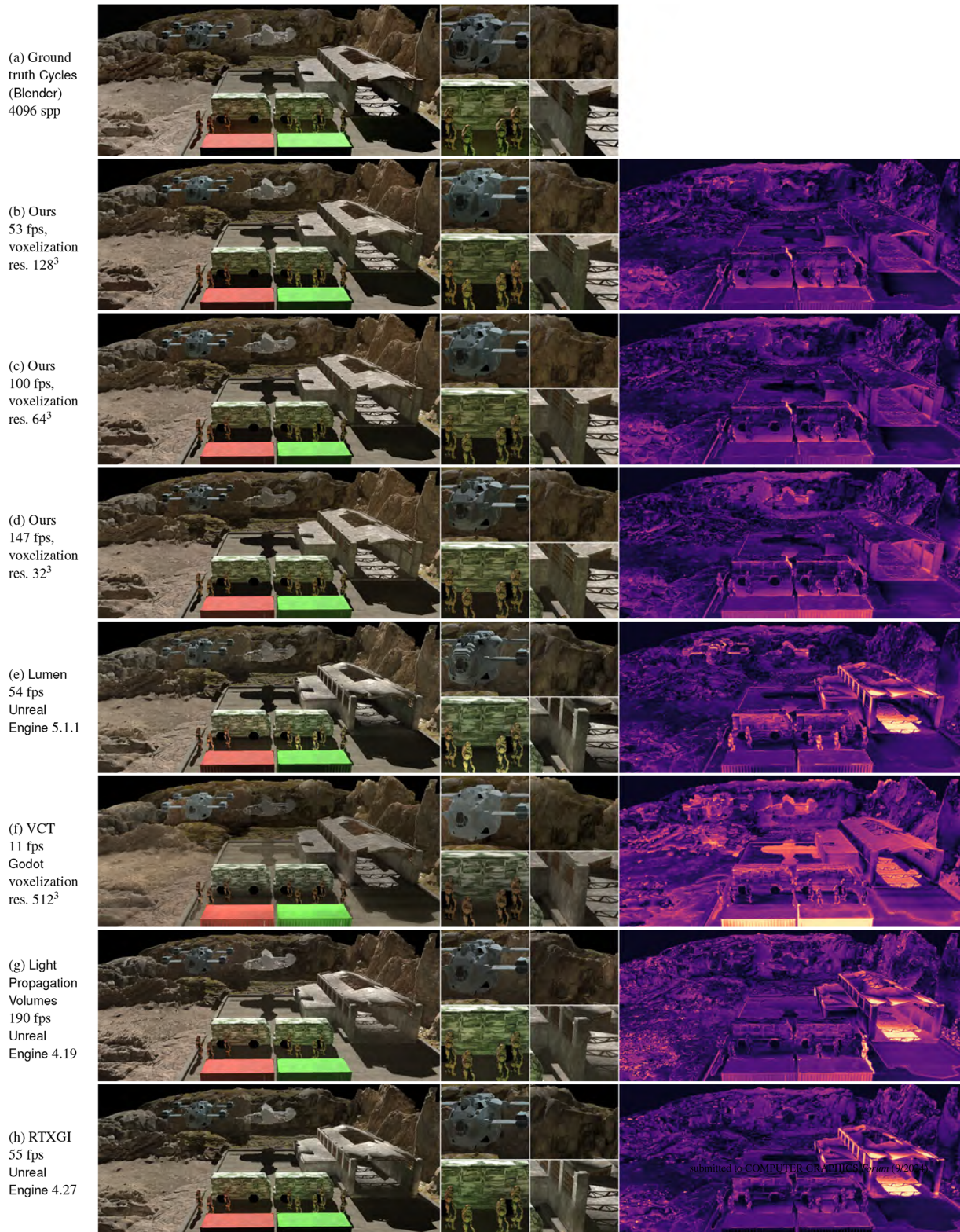
Figure 10: Original images from Figure 8 not using the Enhanced Image Colour Transfer method [JR21]. The rightmost column shows the difference with the ground-truth rendering using NVIDIA's FLIP [ANAM*20] tool.
