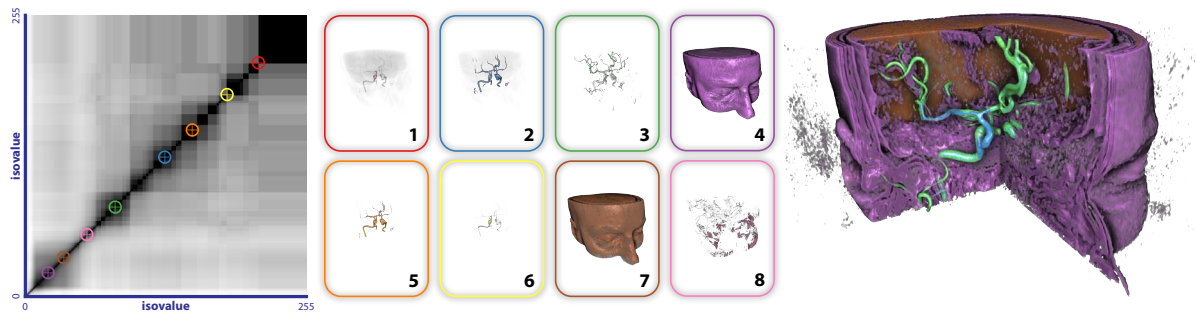
Figure 7: Representative isovalue selection algorithm applied to an MRI angiography data set. The isosurface similarity map is shown on the left and the eight most representative isovalues are marked. The corresponding isosurfaces are depicted in the middle section numbered from one to eight with decreasing relevance. The image on the right shows a cutaway view of the data set classified according to maximum similarity with the eight isovalues.
