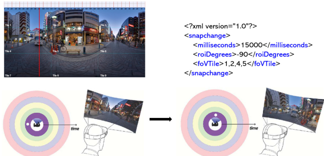
Figure 2: Top left: Identification of the ROI targeted by the snap-change. Top right: Description of the list of snap-changes over the video as an XML file. Bottom: FoV re-positioning in front of the targeted ROI by the snap-change.
