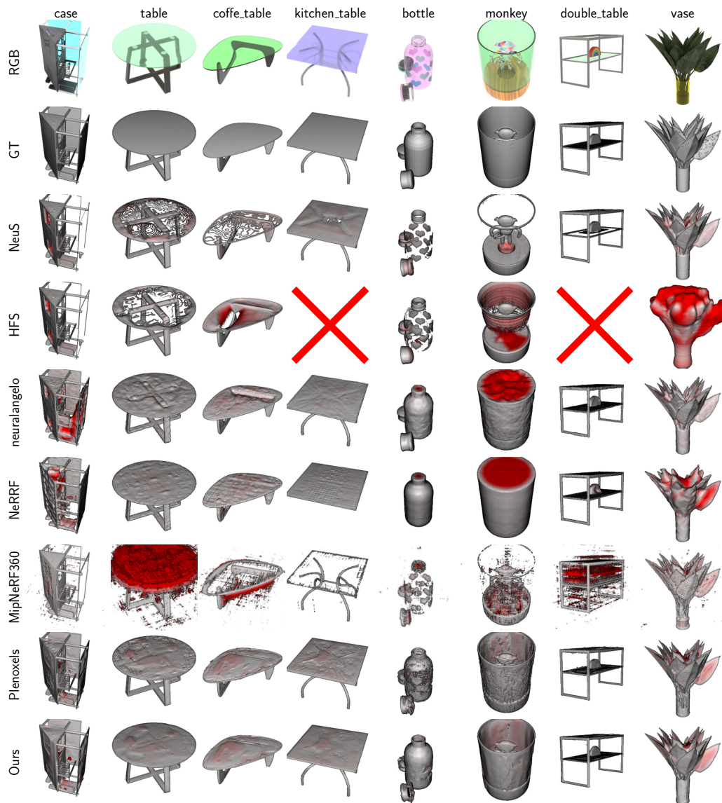
Figure 3.6: Qualitative evaluation on Translucent datasets. Our method can properly recover the translucent surfaces missed other methods.
