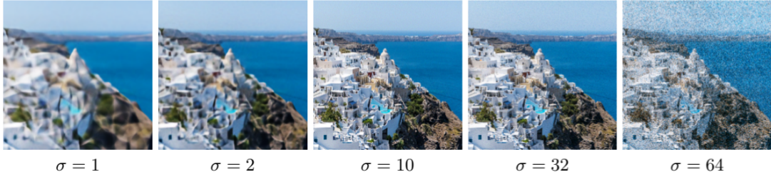
Figure 2.6: 2D image fitting with positional encoding of different frequencies Gaussian-based positional encoding [106] is applied to fit a 2D RGB image with a small MLP, where \sigma indicates the frequency of the encoding. Higher frequency can significantly improve the level of details learned in the MLP, but using a value that is too large can also lead to over-fitting. Figure by Tancik et al. [106].
