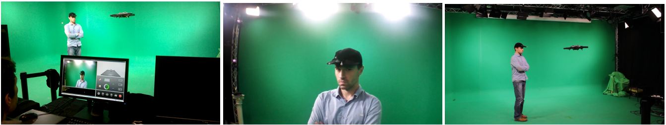
Figure 1: Drone autonomously filming an actor given a specific cinematographic command.
