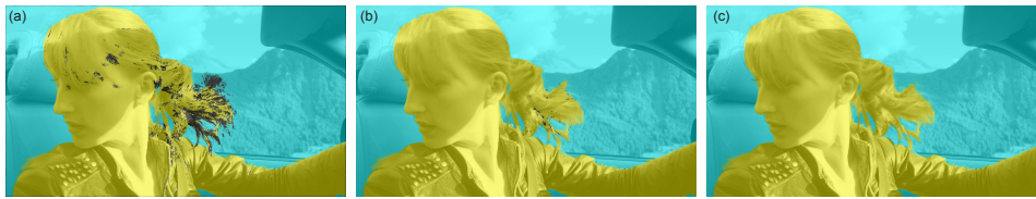
Figure 7: Final propagation result. The initial propagation's (a) holes due to incorrect optical flow are partially filled by propagating through straight motion paths (b). Next, any remaining holes are filled with a final spatial propagation pass (c).
