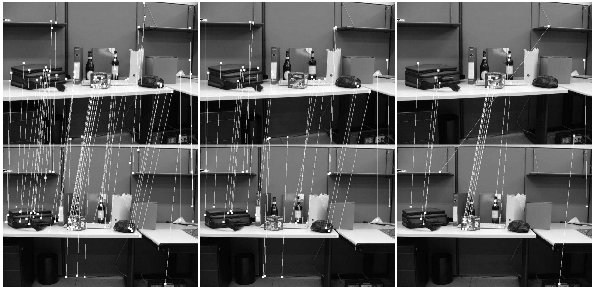
Figure 3: Results for a 5-frames image sequence. Correct matches between first (top) and third (bottom) frame. Left: S-SVD. Centre: C-SVD. Right: S-DIST. Note that one of the matches in the left image is a wrong match that appears to be consistent with the epipolar geometry.
