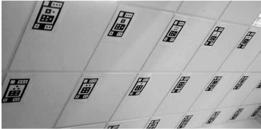
Figure 1: A room ‘instrumented’ with ceiling-mounted VPS fiducials
