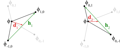
Figure 2: Linearity measure (6) illustrated in 2D: \mathbf{d}_i = \frac{1}{2} (\phi_{\mathbf{e}_i} + \phi_{-\mathbf{e}_i}) - \phi denotes the deviation from mean term (Laplace), which vanishes in a perfectly linear neighborhood. The magnitude of the "spread" \mathbf{h}_i provides the baseline for a relative error.
