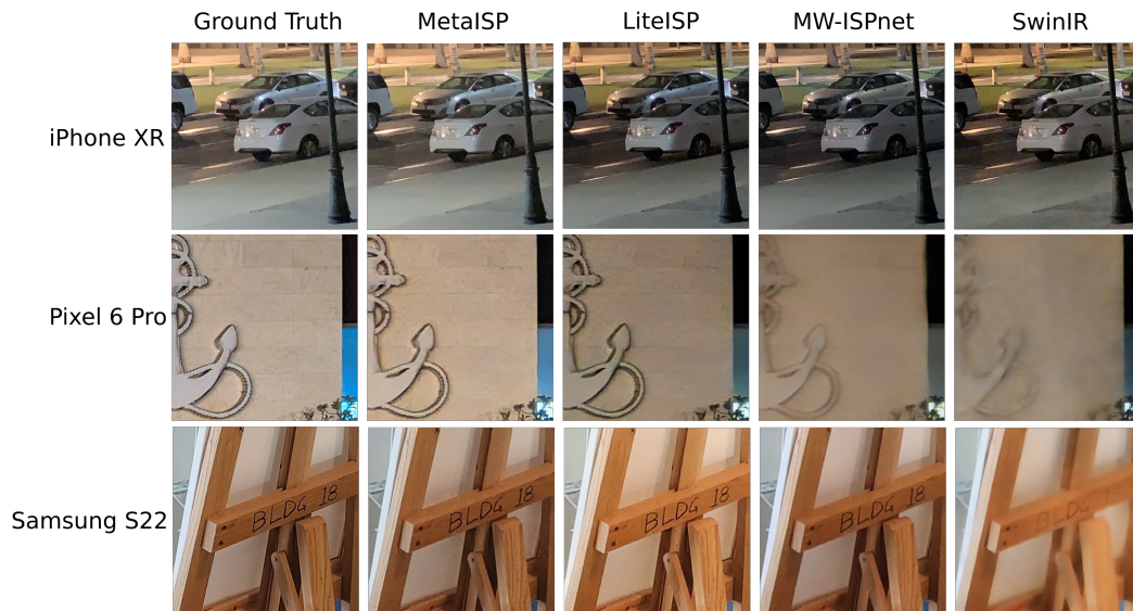
Figure 3: Patch-wise comparison between the different methods and the ground truth. The images mainly represent challenging scenarios such as indoor and night scenes. Our model can accurately reproduce the color appearance of each target device. The alignment strategy described in the supplementary effectively avoids blurry effects that may be observed in SwinIR, resulting in sharper and more visually pleasing results. On the other hand, LiteISP does not suffer from blurry effects but struggles reproducing the color perception.
