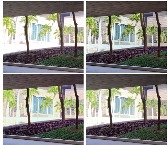
Figure 5: Zero-shot processing of images from new devices. MetaISP generating different interpretations from a Xiaomi C40 input without additional training. Top-left Xiaomi C40 (input, top-right simulated Pixel 6 Pro, bottom-left simulated S22 Ultra and bottom-right simulated iPhone XR. Please zoom for more details.
