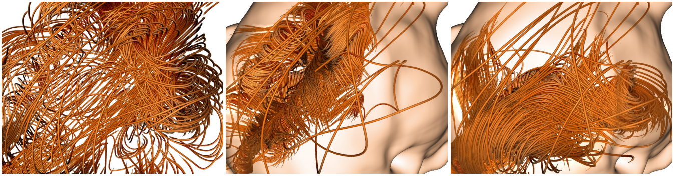
Figure 8: Comparison of importance-based density control as proposed by Kanzler et al. [KFW16] (left) and our brush based visualization (center and right). The vortex at the bottom of the image is not covered by Kanzler et al. but can be brought out using our brush (right).
