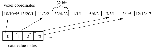
Fig. 3. Value-sorted array structure: All voxels are sorted according to data value and their position in space is stored in an array. An additional index points to the first voxel in the array for each possible data value
