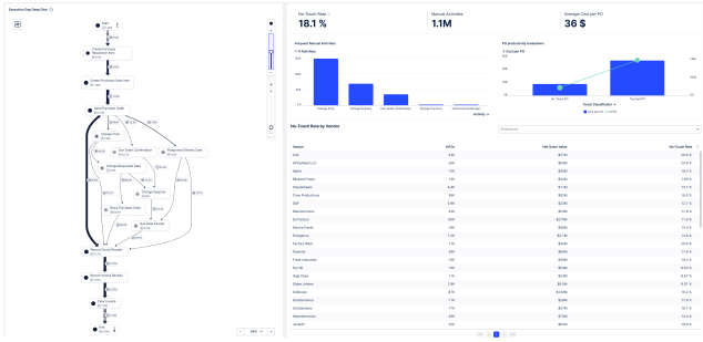
Figure 4: Multiple coordinated views in Celonis. On the left, Process Explorer graph shows process data with connection thickness encoding the number of cases. Top right view shows the Bar Chart depicting frequencies of activities categorized by event type. Table on the bottom right shows a list of values sorted by KPI.
