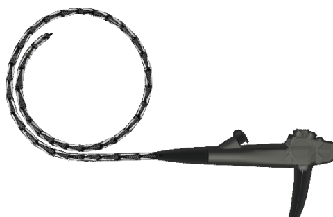
Figure 8: A view of the endoscope model used in the prototype (model source: 3d Molier International, TurboSquid) including the bones that we added to the shaft during the rigging process
