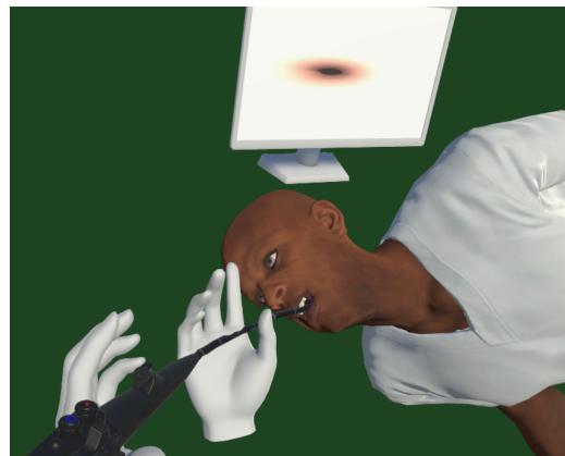
Figure 5: Example view from the HMD. The endoscope has been advanced into the patient and the view from the endoscope camera displayed on the monitor. The scene will be enhanced once the operating theatre furniture has been included.
