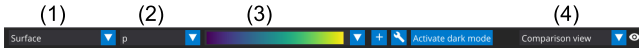
Figure 7: Toolbar to select visualization (1), pick calculated field (2), select and add color maps (3), and change current view (4).
