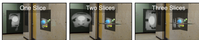
Figure 3: Images from the HoloLens showing the operator selecting one, two and three slices from the MRI set that are then refreshed in both the 3D rendering window (right side) and the 2D virtual window (left side).
