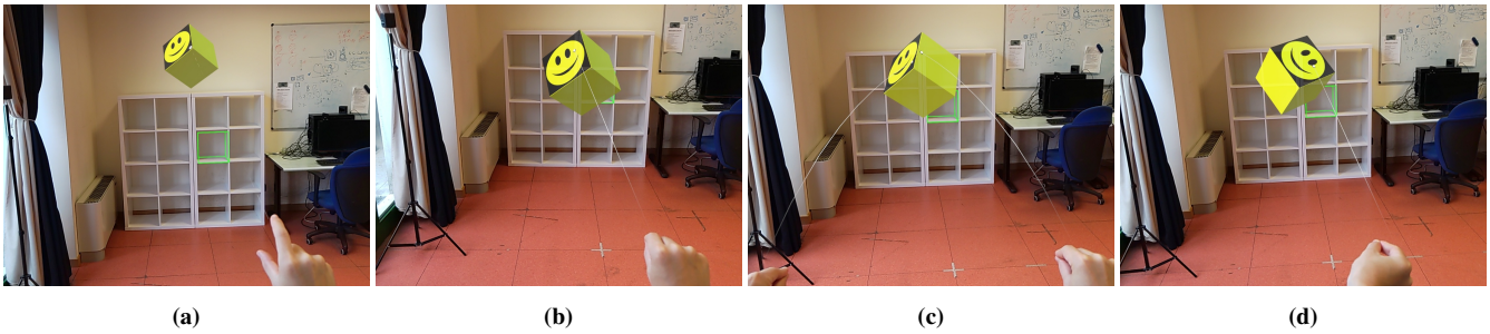
Figure 2: Task performed with the default MRTK 2 implementation. (a) the object is selected. (b) the object is translated by mapping the hand displacement on the object’s one. (c) Scaling is performed with the second hand by pinching and mapping the ratio between the hands’ distance and the initial one over the scale factor. (d) The rotation is directly mapped from the dominant hand pose, or, in case of activation of the second hand, can be controlled by changing the orientation of the line joining the two hands.
