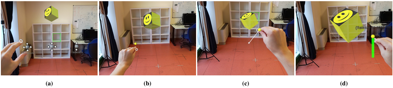
Figure 3: Task performed with the desktop-inspired option: after the selection, mid-air buttons appear (a) allowing the separate control of translation (b), rotation (c) and scaling (d) with remapped single-hand translation.
