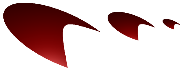
Figure 1: The proposed method of clipping splats allows to adapt them to curved edges regardless of the number of samples of the model and the distance from the viewer. The clipping curve is sampled in pixel precision.
