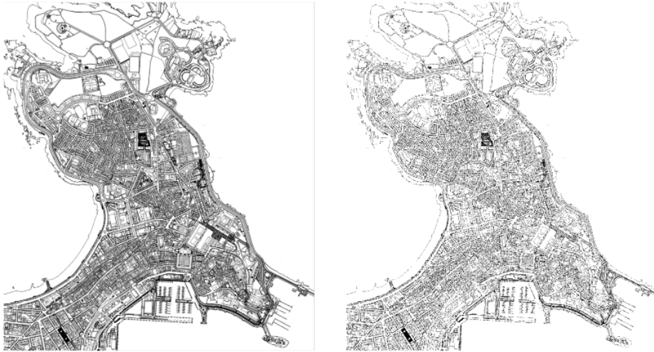
Figure 9: Comparison between line (left) and polygon (right) primitives for rendering of thin lines.
