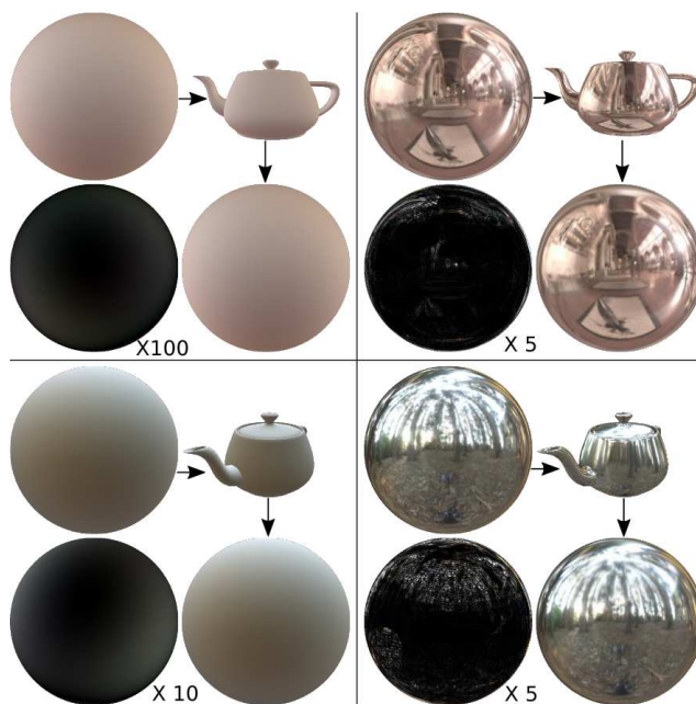
Figure 6: Reconstruction results for diffuse (left column) and reflection (right column) shading, using Galileo (top row) and rnl (bottom row) light probes. Each quadrant shows the reference prefiltered environment, along with the rendering of a 3D teapot assuming distant lighting and no shadowing or inter-reflections. The teapot image is then used to reconstruct the prefiltered environment using either the method of Section 3.1 or 3.2, and a boosted absolute color difference with the reference environment is shown.
