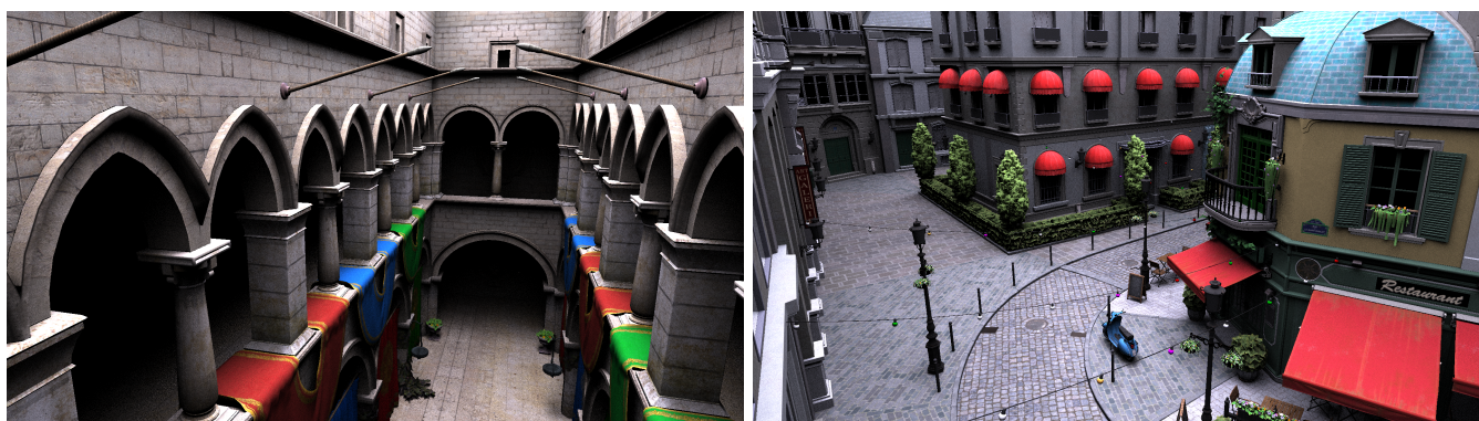
Figure 1: Rendering results of ray-traced environment lighting with our proposed precomputed discrete visibility fields. Left: Crytek Sponza (262 K triangles), 128 spp, 15.95 ms. Right: Amazon Lumberyard Bistro (2.8 M triangles), 64 spp, 33.67 ms.
