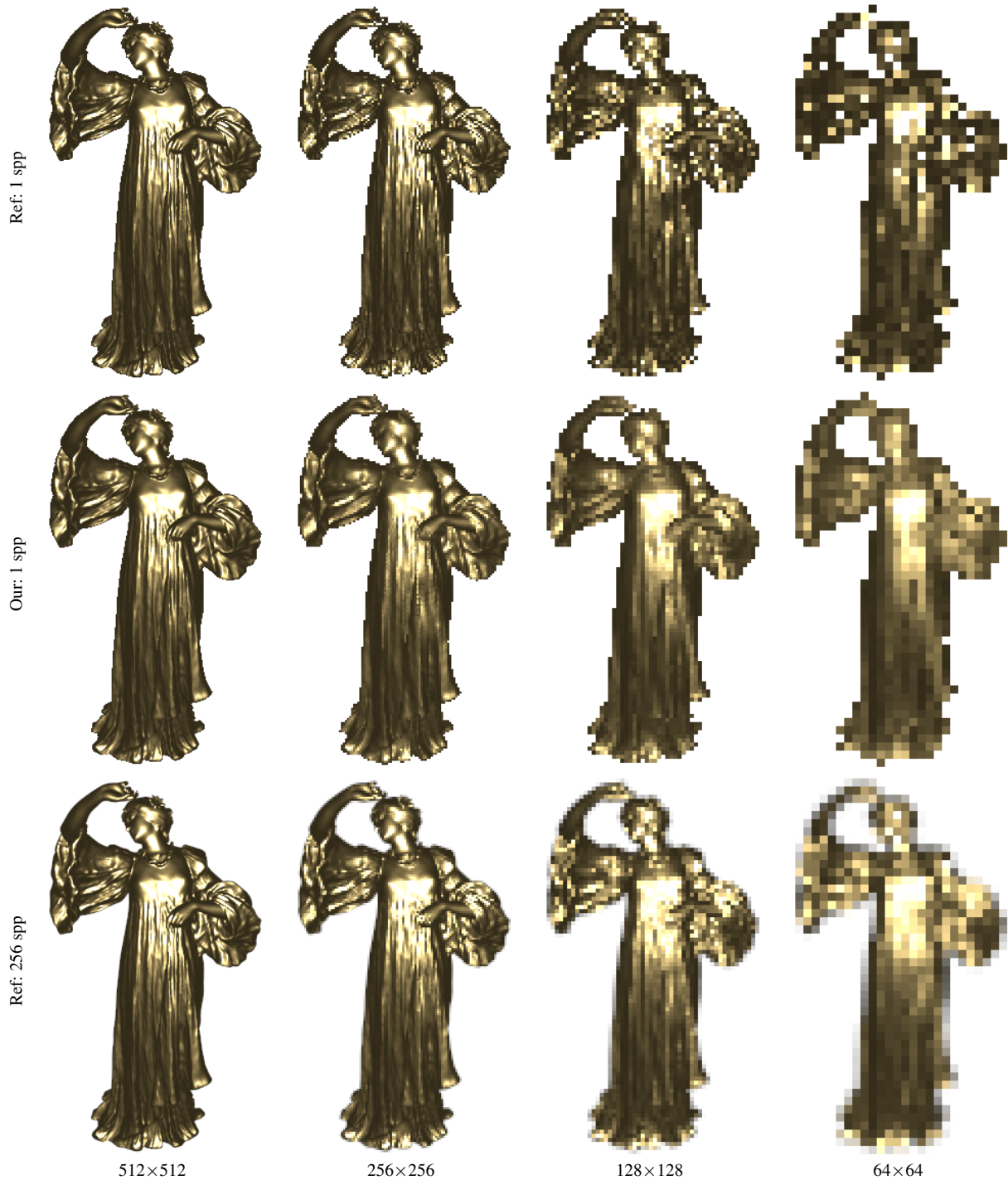
Figure 12: We perform shape and appearance prefiltering by optimizing for a particular rendering resolution. Here, we show our results for four different resolutions. As expected, geometric details and shading are smoothed as rendering resolution decrease. Top: The reference dancer model rendered at 1 spp, note the aliasing. Middle: Our optimized model with prefiltered shape and appearance rendered at 1 spp. Bottom: The reference dancer model rendered, with antialiasing, at 256 spp.
