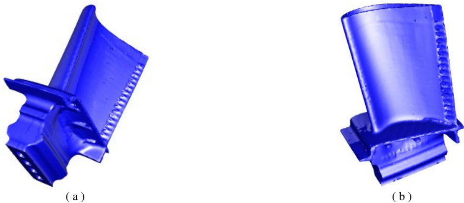
Figure 5: Turbine Blade: Reconstructed mesh with GBF method ( a ) Back view; ( b ) Front view.
