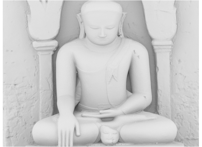
Figure 3: Part of Eim Ya Kyaung resampled (2.9% of the 1.3 billion original points remaining) and reconstructed using [BL17].
