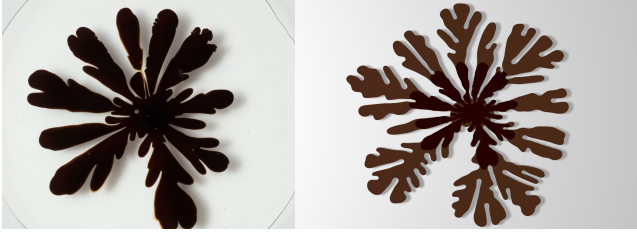
Figure 9: “Continuing” an experimental Hele-Shaw flow. (left) Photograph by Antony Hall. (right) Our evolution starting from the boundary curve of the photograph.
