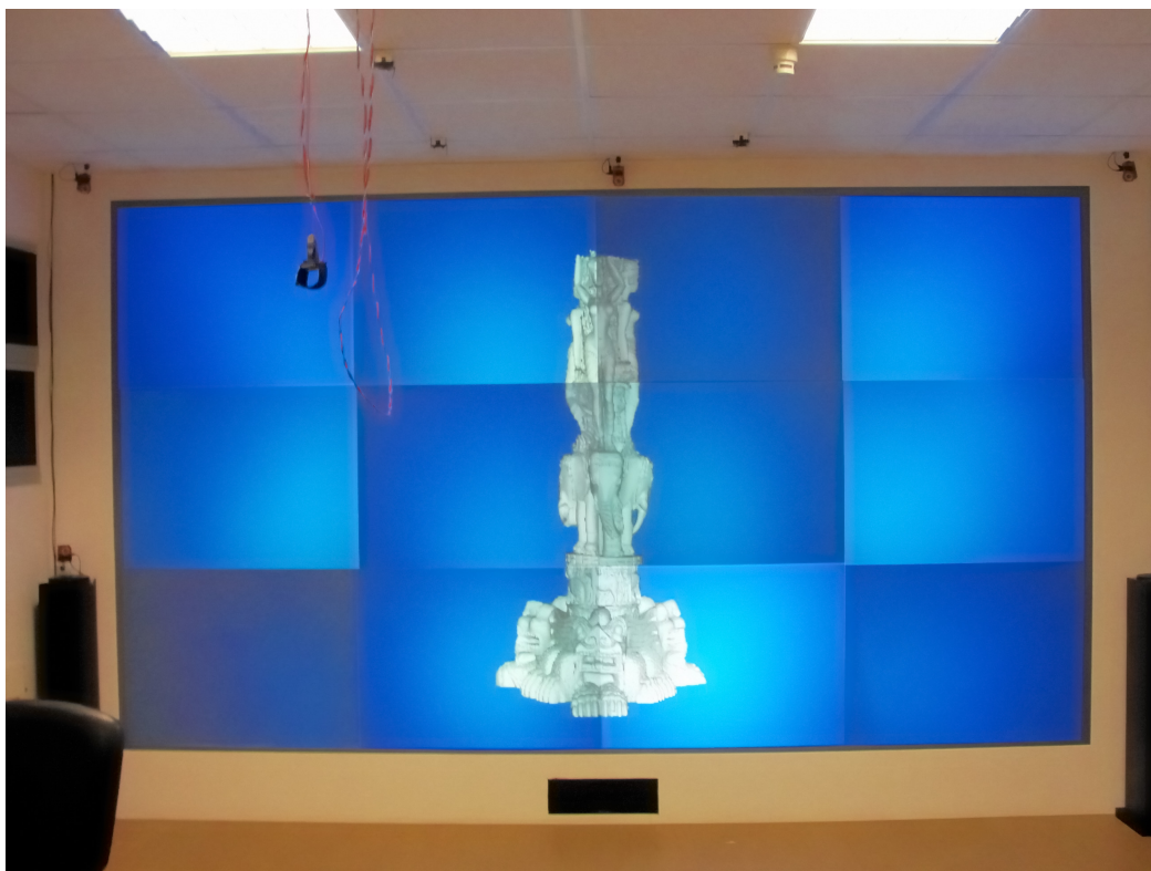
Figure 10: Rendering of the Thai Statue (10 Mtri) on the 4.00m \times 2.25m display wall. The hardware powering this application consists of a ray tracing cluster of twelve machines with the screen compositor server running on a separate machine.
