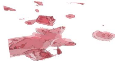
Figure 5: Five isosurfaces corresponding to resistivity values 80%, 85%, 90%, 95% and 100%.
