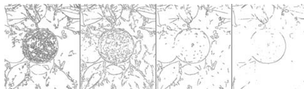
Figure 4: Edges by Canny, Nalwa, Bergholm and Iverson algorithms.
