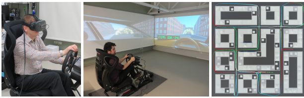
Figure 1: Equipment setup. Left: HMD. Centre: CAVE. Right: A city layout with the path taken by one of our subjects (the colour shading indicates time taken).
