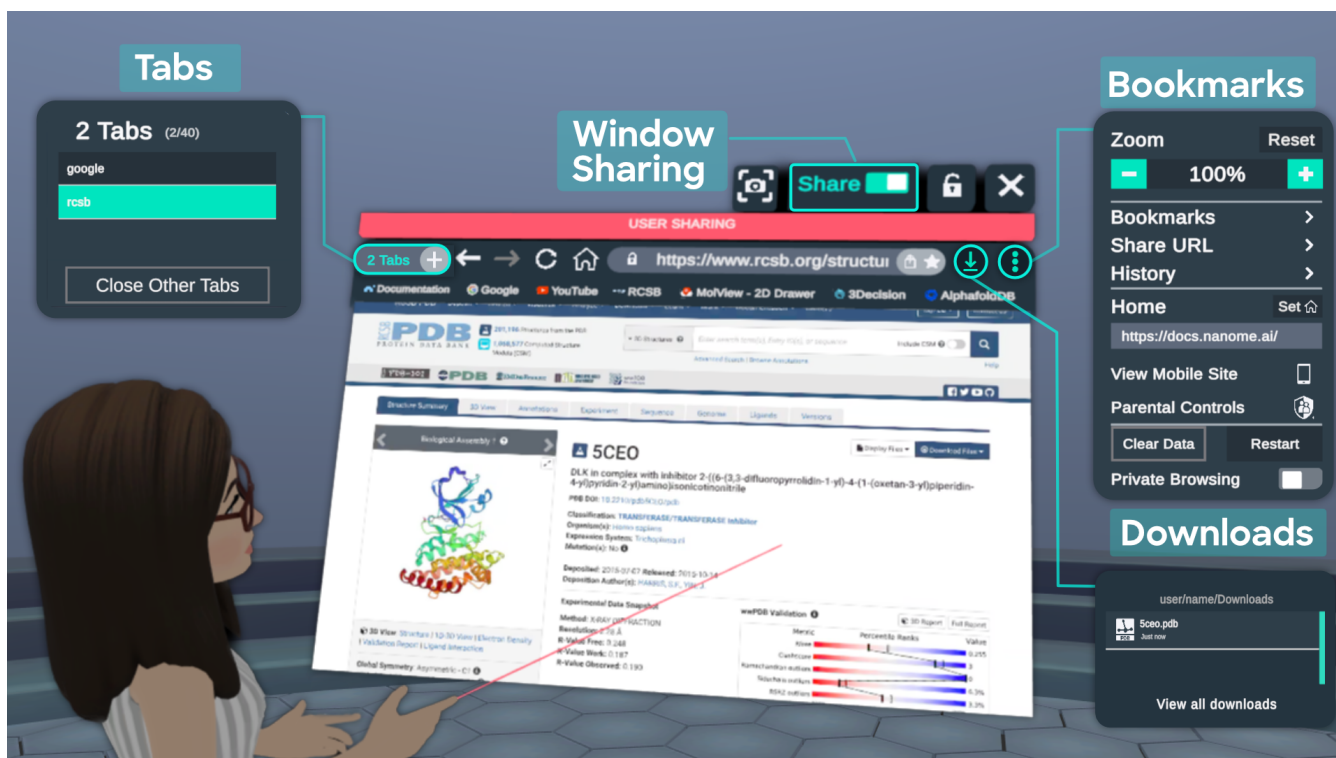
Figure 2: In-VR web browser. The user has access to a fully functional web browser in VR. Specialized buttons on the browser window open panels that allow the user to navigate through different tabs, save bookmarks, retrieve browsing history, share URLs, launch downloads, and open downloaded files.
