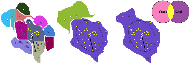
Figure 4: Clustering based on different kernel sizes. Left: too small kernel, s(\phi) = 0.63 ; Middle: the optimal size of the kernel, s(\phi) = 0.72 ; Right: too big kernel, s(\phi) = 0.64 .
