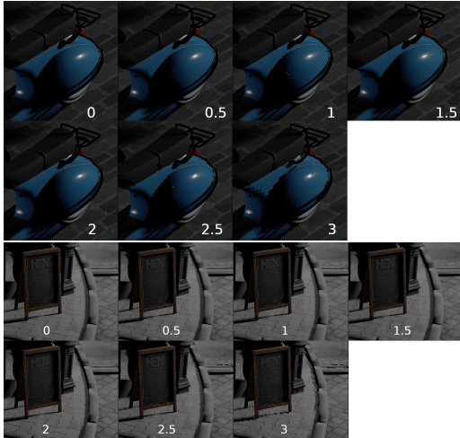
Figure 2: Bias comparison details for Bistro Exterior [Lum17]: for a cache bias of up to 1.5 visual quality is close to identical to for resolution caching. With a bias of 2.0 and more artifacts around object boundaries and shadow boundaries become visible.
