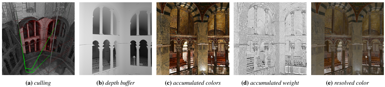
Figure 5: Our rendering (extended from [BHZK05]) consists of four passes. First, a compute shader performs culling of splat chunks and populates a draw call buffer (a). Then, a visibility pass renders slightly pushed back splats to allow accumulation within a small margin (b). The attribute pass uses additive blending to accumulate weights and weighted colors in two render targets (c,d). Finally, a post-process resolve pass computes the properly blended output color (e). The stripe pattern in the accumulation targets is an artifact of the input splat distribution.
