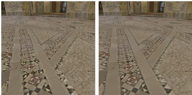
Figure 6: Instead of rendering only the front-most splat fragment, we use the multi-pass rendering of [BHZK05] to average the contribution of all splats within a certain margin. The figure shows an example without margin (left) and with a 2 cm one (right). The margin is essential for hiding the underlying splat structure.
