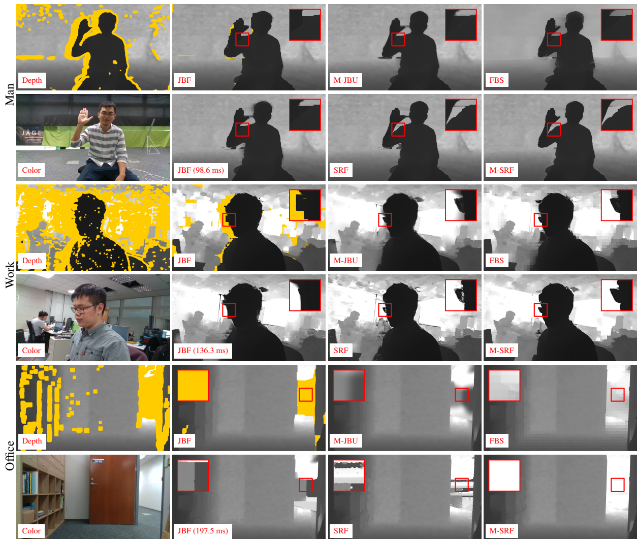
Figure 13: Equal-time comparisons of real data captured by Intel RealSense D435. Same as Figure 9, we allocate 15 milliseconds for the single-pass methods and 7.5 milliseconds for the multi-resolution ones. We also list the results of single-pass joint bilateral upsampling with large enough kernels for filling all holes and the ones of fast bilateral filter (FBS) for quality comparisons. Our method reconstructs depth maps significantly better than other methods by avoiding to oversmooth the depth boundaries.
