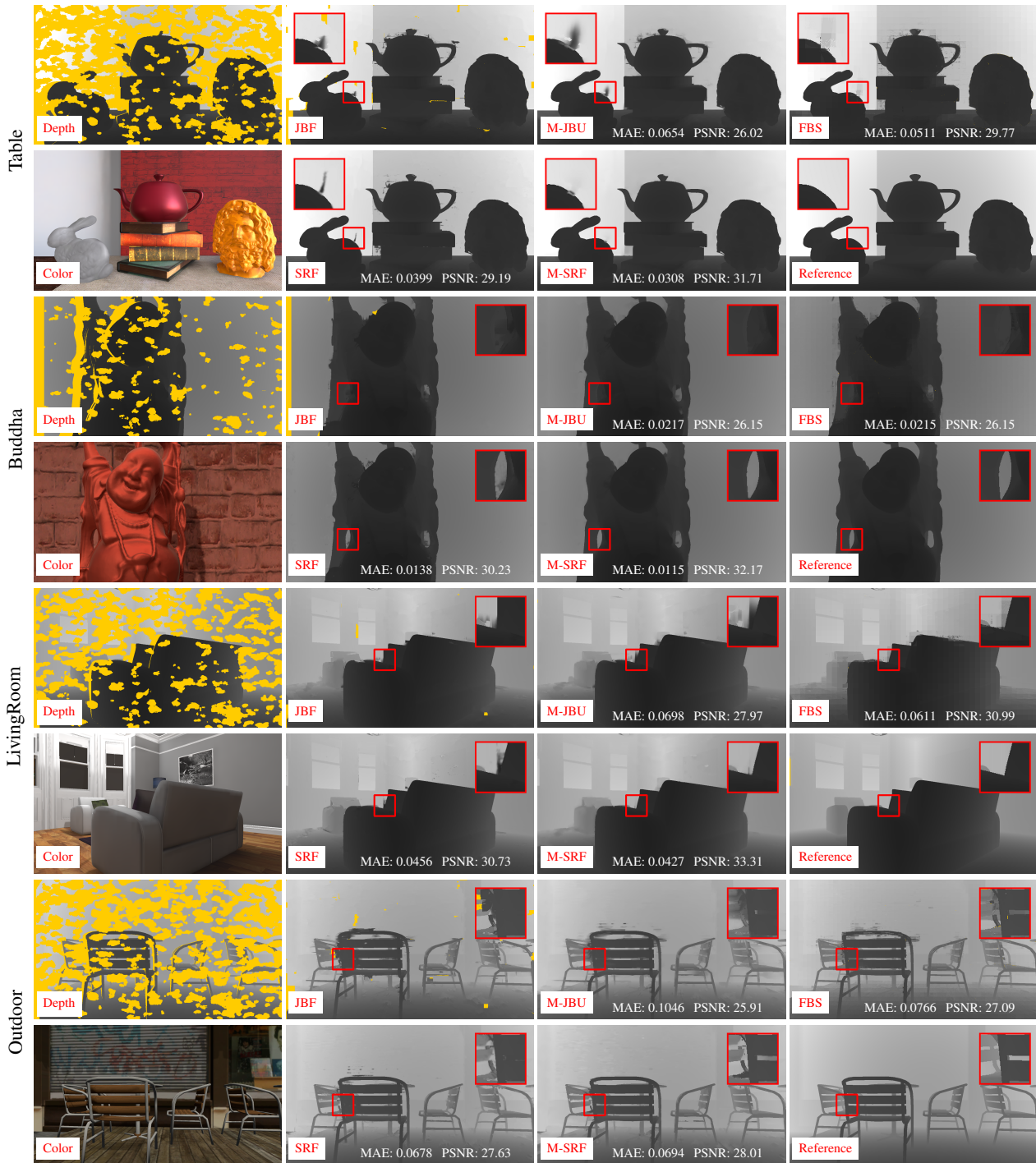
Figure 9: Equal-time comparisons for four synthetic RGB-D scenes: Table, Buddha, LivingRoom, and Outdoor. For each scene, the first column shows the input depth map (top) and the color image (bottom). In the depth maps, yellow pixels represent missing depth values. The second column shows results of single-pass joint bilateral upsampling [KCLU07] (JBF) and our method (SRF), while the third column shows multi-resolution versions (M-JBU [RSD*12] and M-SRF). We allocate 15 ms for the single-pass methods and 7.5 ms for the multi-resolution ones. The Python version fast bilateral solver (FBS) [BP16] takes about 0.3 to 0.5 second, running on CPU. Its results are still listed for quality comparison. The peak signal-to-noise ratio (PSNR) is denoted for each depth map. In the given time budget, JBF fails to complete all missing regions (therefore, we do not measure its error), while M-JBU and FBS oversmooth depth boundaries. Our method demonstrates significant improvements both numerically and visually, and shows 0.92 to 6.02 dB of PSNR gain over previous methods.
