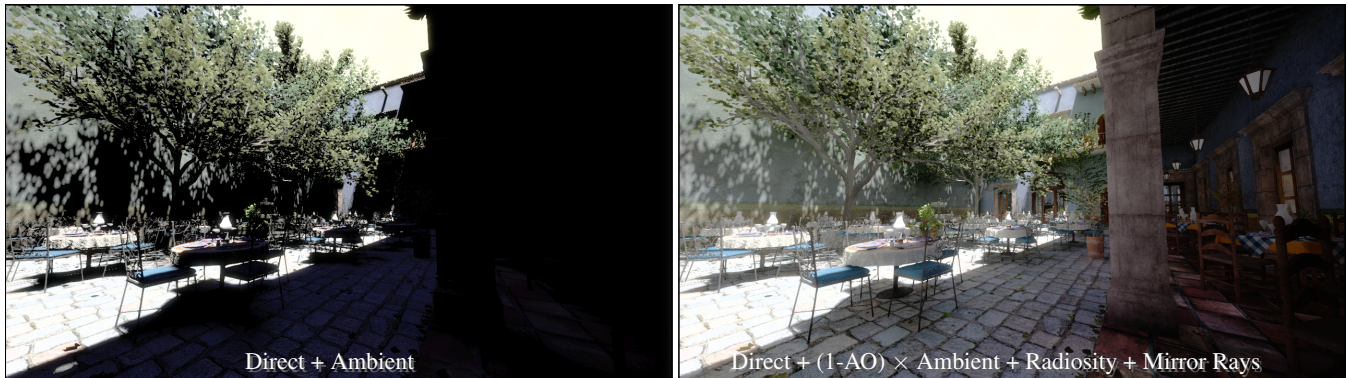
Figure 1: Left : Direct and hemispherical ambient illumination in San Miguel (6.5M triangles, 968 draw calls). Right : Direct lighting, approximate radiosity, mirror reflections, and AO computed from a two-layer Deep G-buffer in 5 ms at 1080p on NVIDIA GeForce 980. The G-buffer was generated in a single 5.8ms geometry pass. See our evaluation section for faster results on more game-like scenes.
