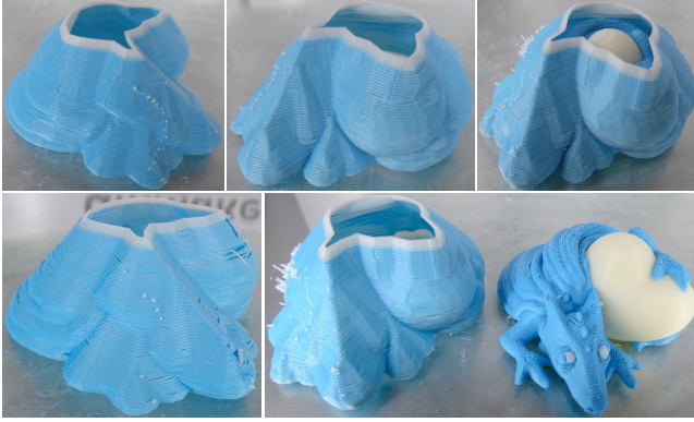
Figure 13: Top. Back and front of a simple enclosure printed alone. The enclosure is two filaments thick and requires no support structure. Each other layer is of a different color. Top right. Same protective enclosure printed with the dual-color dragon model inside. Bottom left. This print is a single filament thick. Bottom right. The dragon has been taken out of its enclosure.
