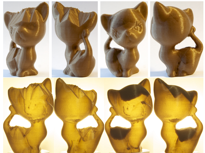
Figure 6: The kitten. Top-left. Front and back view of the cavity. Top-right. Front and back view of the hollowed kitten. Bottom. Same as above with back light. The cavity is completely empty, while the hollowed kitten is filled between its inner cavity and its surface (eq. (10)).
