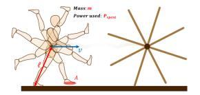
Figure 3: Yoyo-man (@Laumond) with our input parameters in red, enabling to compute the speed value v (norm of velocity).
