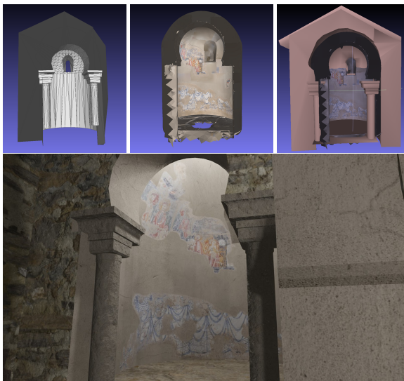
Figure 12: Top: the architectural model (left) and the photogrammetric model (center) are aligned using ICP (right). The bottom image shows the result of transferring the paintings onto the procedurally textured model.
