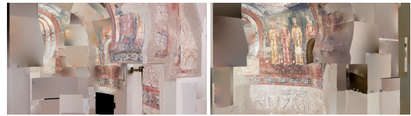
Figure 9: When the changes in illumination depended on the orientation of the different parts of the surface, we divided the texture into different layers that were later combined to achieve well-exposed textures. The texture layer for windows, arch, and the front wall is shown on the left, while the texture layer for the interior of the apse is shown on the right.
