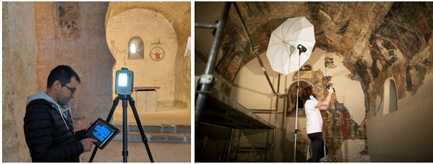
Figure 2: The acquisition of the data was a two-step process for the three locations: we captured the surface using a laser scanner (left) and the appearance of the paintings using a specific photographic setup (right).
