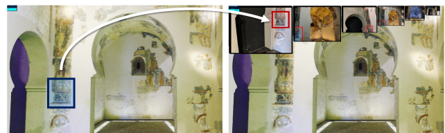
Figure 10: When the user selects a RoI (left) the application selects, groups and shows the relevant images; the overlapping part is outlined in red (right) to facilitate the localization of the RoI within the thumbnails.
