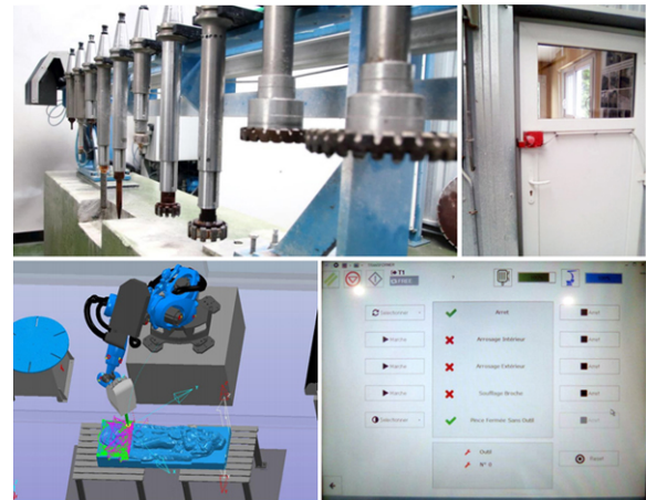
Figure 4: Machining tools, door with a security system, 3d simulation and watering system whose parameters must be configured for the milling process
