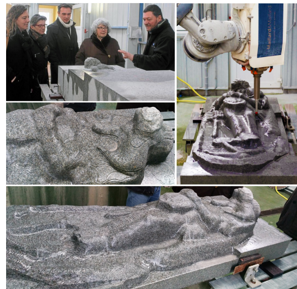
Figure 5: Different steps of milling by the robot
