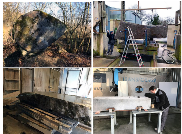
Figure 2: Extraction and rough cutting of the granite ball
