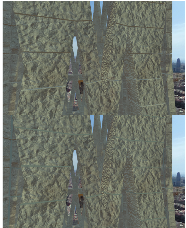
Figure 7: On the top, an example of the temple with gaps between stones. On the bottom the same image with the mortar filling simulation.
