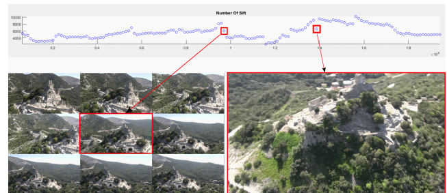
Figure 1: Two examples of frames selected during the pre-filtering stage. Top: the graph of the number of SIFT extracted for each selected frame. Left: a frame associated to an abrupt change of position and direction of view. Right: a blurred frame.
