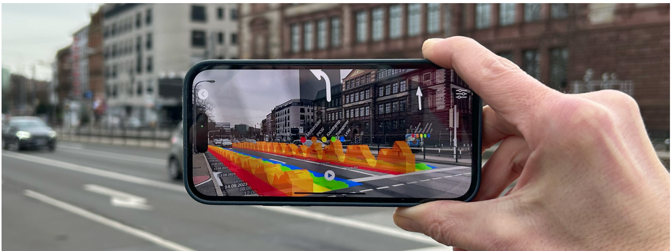
Figure 1: Hand-held mobile device displaying a grouped area chart embedded onto the street visualizing the progression of traffic by type for two lanes. Time labels are shown along their axis, with arrows and legends hovering slightly over-head.
