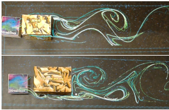
Figure 3: Visualizations of the flow patterns created when using different obstacle sizes. Top: small obstacle, bottom: large obstacle.
