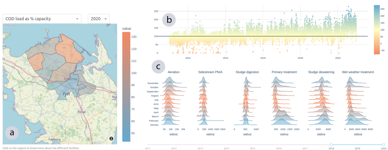
Figure 1: Overview of our system: (a) map of Fyn shows areas connected to Vandcenter Syd's treatment facilities, (b) scatter plot shows ratio of energy produced versus consumed at the Ejby Mølle WRRF, and (c) ridge line plot shows distributions of energy consumption by type at the Ejby Mølle WRRF, by month.
