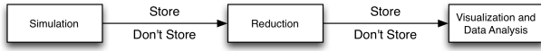
Figure 4: A simple workflow that begins with a simulation, extracts a feature and performs visualization and data analysis on that feature with the decision to store or not store data between each processing element.
